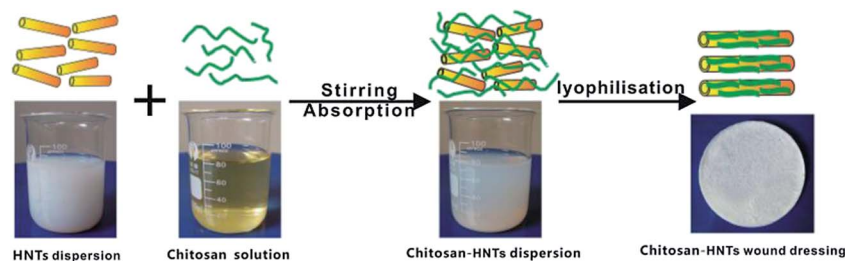
Fig. 1 Schematic representation of the preparation of chitosan–HNTs composite sponges.
