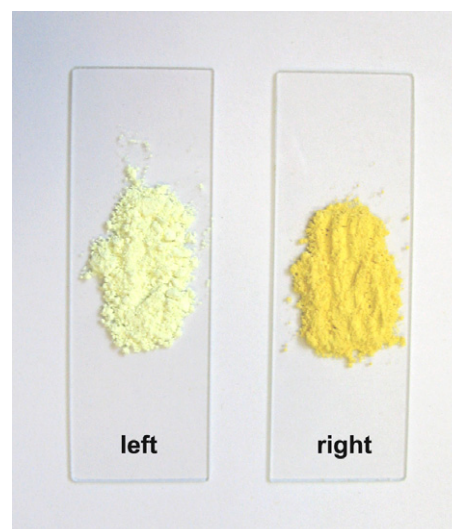
Figure 6. Photos of the HNTs/BBT complex (left) and the heat-treated HNTs/BBT complex (right).
