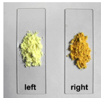
Figure 5. Photos of the HNTs/EPB mixture (left) and heat-treated HNTs/EPB complex (right).
