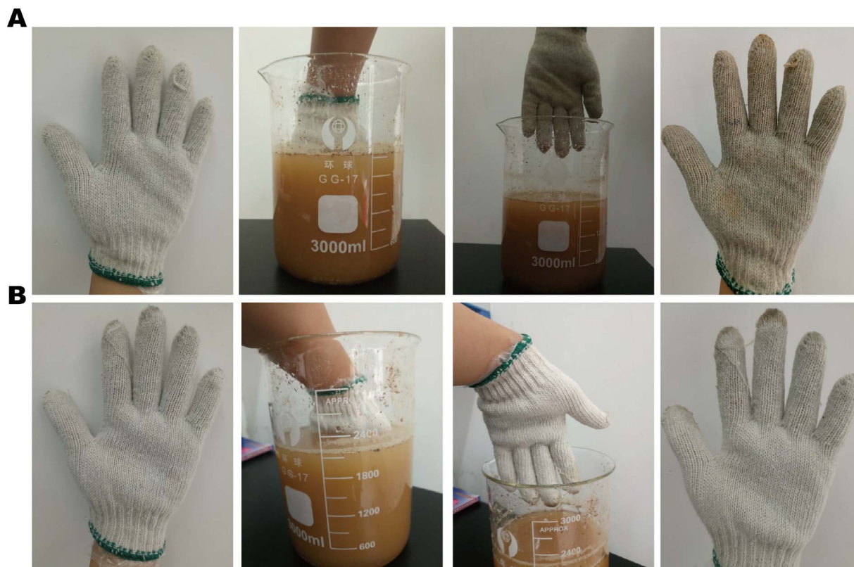
Fig. 9. Photos of uncoated (top) and hydrophobic HNTs coated (bottom) cotton gloves before and after being soaked in mud solution.
